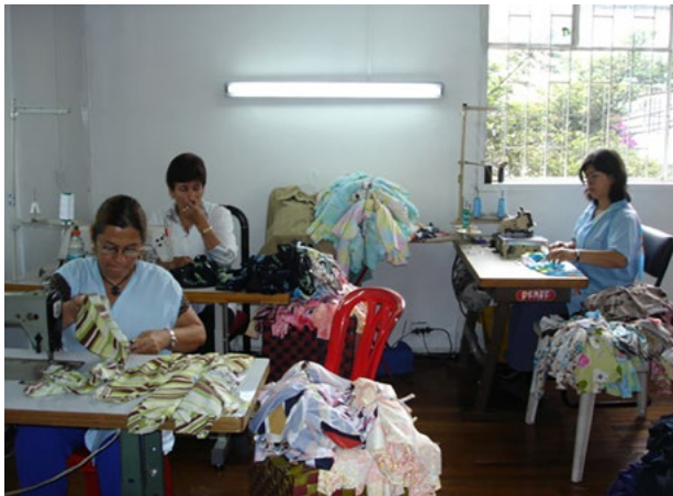
Figure 5. The employees sewing in an assembly line process. You can see how the fabric pieces pile up, indicating that the garments are reproduced and the operations are repeated.
